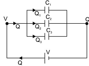
**Ex.18** Three initially uncharged capacitors are connected to a battery of 10 V in parallel combination find out following
