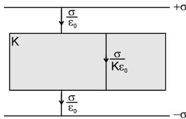
The total electric field produced by bound induced charge on the dielectric outside the slab is zero because they cancel each other.
