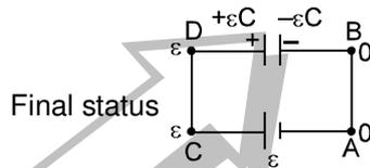
Let potential at point A is 0, so at B also 0 and at C and D it is  $\epsilon$ . finally, charge on the capacitor
