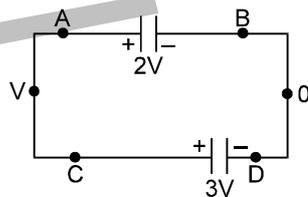
Let potential of B and D is zero and common potential on capacitors is V, then at A and C it will be V
