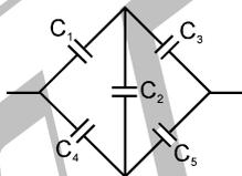
The given combination can not be simplified by series or parallel combination such a combination is solved by using kirchhoff's law and other techniques. A special case of this combination is Wheatstone bridge.
