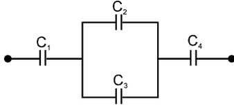
The given combination is neither a series nor a parallel combination but C<sub>2</sub> and C<sub>3</sub> are in parallel and that is in series with C<sub>1</sub> and C<sub>4</sub>.
