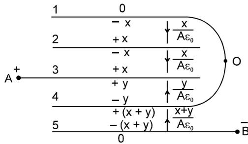
$$C = \frac{Q}{V} = \frac{x+y}{V_{AB}}$$
