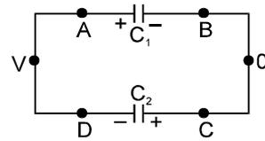
**Ex.11** Find out the following if A is connected with C and B is connected with D.
