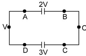
**Sol.** Let potential of B and C is zero and common potential on capacitors is V, then at A and D it will be V
