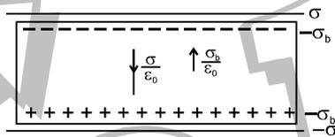
$\sigma_b$  = induced charge density (called bound charge because it is not due to free electrons).
