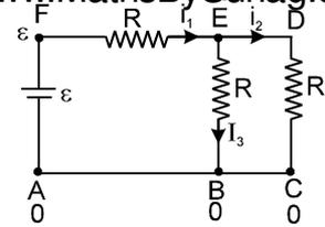
Let potential at A is zero so at B and C also zero and at F it is ε. Let potential at E is x so at D also x. Apply Kirchoff's 1<sup>st</sup> law at point E :
