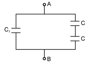
$$C = C_1 + \frac{C_2 C_3}{C_2 + C_3}$$
