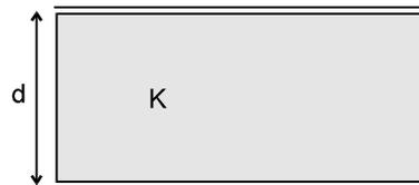
Here capacitance is increased by a factor K.
