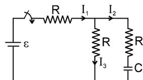
**Sol.** Initially the capacitor is uncharged so its behaviour is like a conductor
