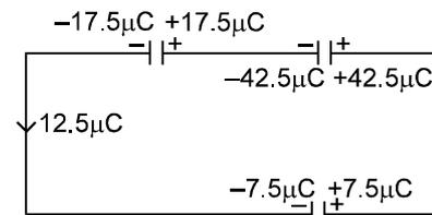
**Ex.15** In the given circuit find out the charge on each capacitor. (Initially they are uncharged)
