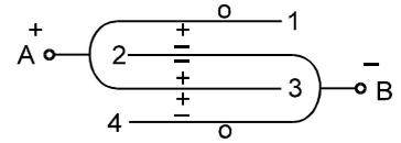
**Ex.46** Find out equivalent capacitance between A and B.
