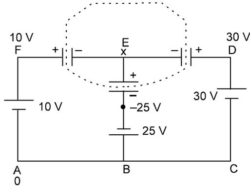
Let potential at A is 0, so at D it is 30 V, at F it is 10 V and at point G potential is -25V. Now apply kirchhoff's 1<sup>st</sup> law at point E. ( total charge of all the plates connected to 'E' must be same as before i.e. 0)
