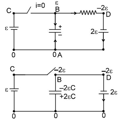
**Ex.8** A capacitor of capacitance  $C$  which is initially uncharged is connected with a battery. Find out heat dissipated in the circuit during the process of charging.
