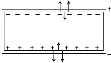
If dielectric is completely inside the capacitor then force is equal to zero.
