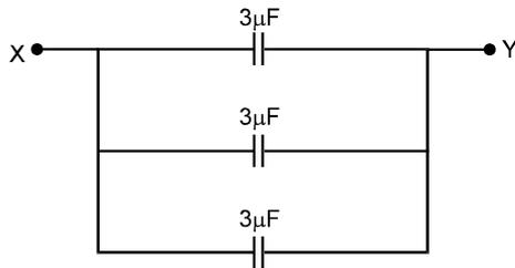
All the three condensers are connected in parallel, hence the resultant capacity
