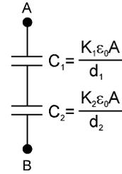
This formula suggests that the system between A and B can be considered as series combination of two capacitors.
