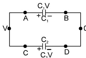
Let potential of B and D is zero and common potential on capacitors is  $V$ , then at A and C it will be  $V$
