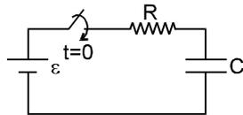
it is given that initially capacitor is uncharged.
